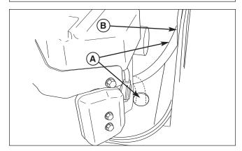
Figure 15. Engine Oil Drain A. Oil Drain Hose
